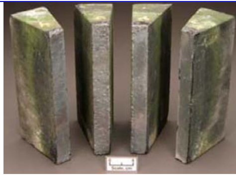
Advanced Refractories For Gasifiers Target is refractory material that lasts years, rather than months
